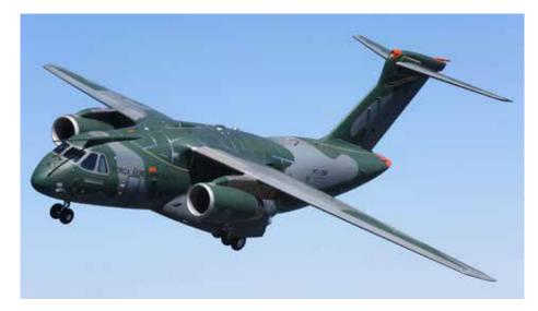
The KC-390 is capable of carrying out various missions, such as transporting cargo, troops or dropping paratroopers, and aerial refueling, search and rescue, medical evacuation and aerial firefighting, in addition to supporting humanitarian missions. The aircraft can transport up to 26 metric tons of cargo at a maximum speed of 470 knots (870 km/h), as well as operate in hostile environments, including from unprepared or
